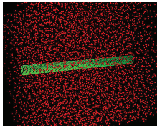
Figure 1. Model of the nanocomposite system (SWCNT in polymer matrix) along the z -axis. For clarity, the connectivity of the beads is not shown.
